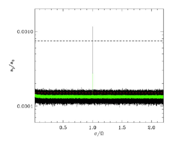
Search for coherent signal, compute single FFT power spectrum, 2<sup>30</sup> light curve bins.
